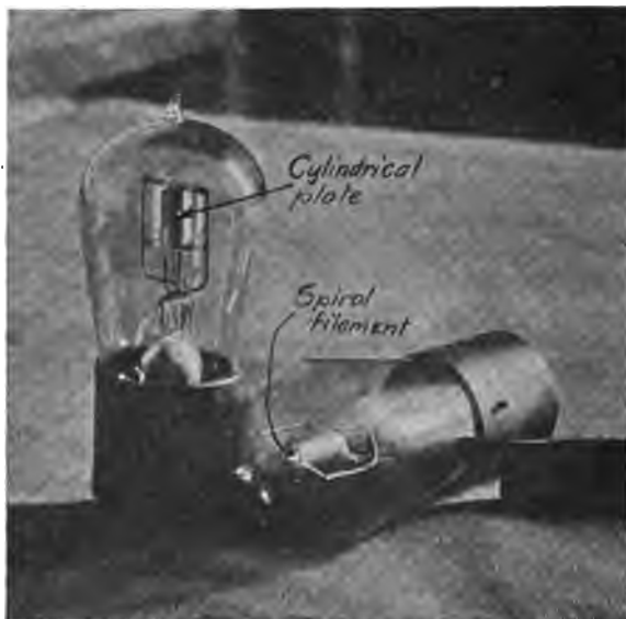
FIG. 8.—Showing the kenotron from which the curves of Fig. 7 were obtained.
